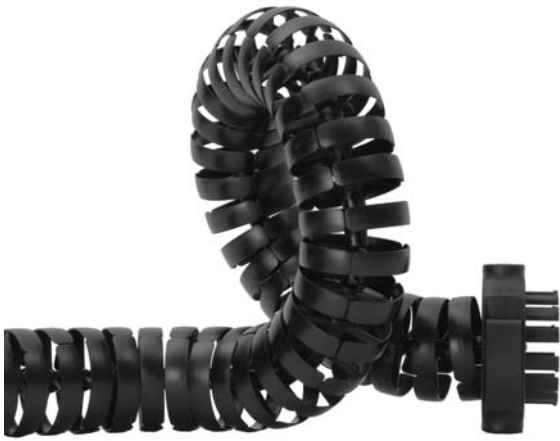
Picture PM0705-02: igus GmbH, Cologne The new highly flexible 3D energy guiding system Triflex R light (igus) doesn't need any additional reinforcements such as continuous steel or bearing ropes.
