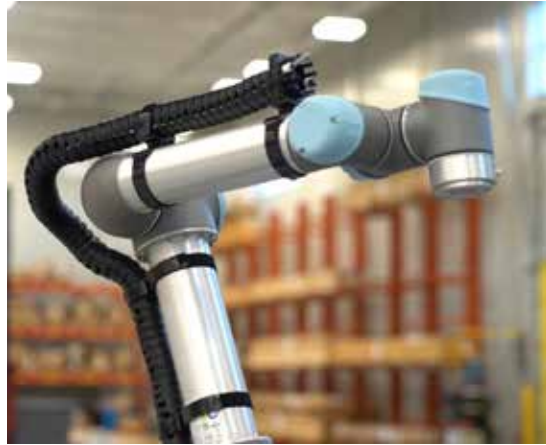
Example of a UR bracket in the igus® test lab
